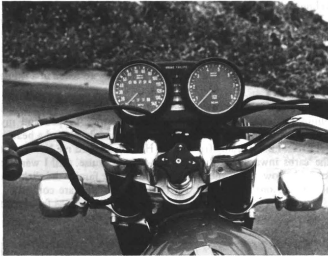
Completely redesigned instrument panel features warning lights and a resettable trip-meter.
