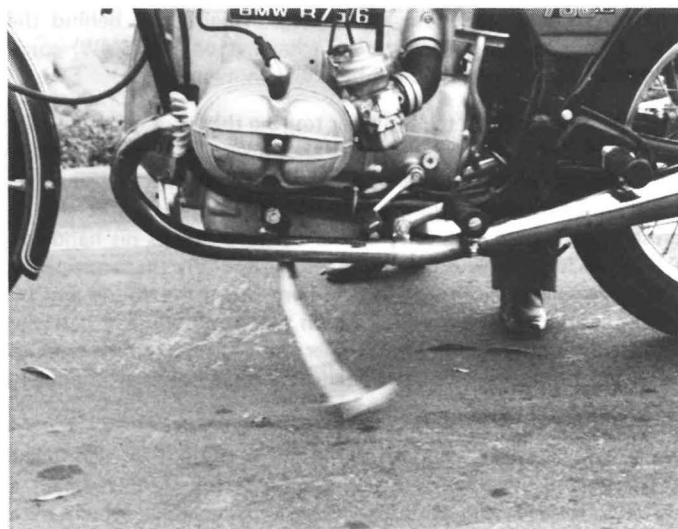
Patti (on opposite side of R75/6) demonstrates the return function of the sidestand.
