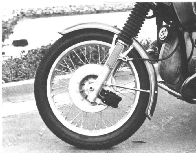
The disc brake features a low-profile caliper housing and out-of-sight, out-of-mind hydraulic reservoir.
