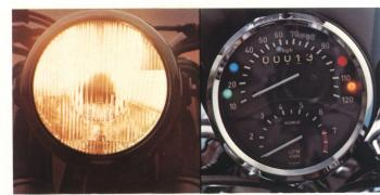
The brilliant Bosch headlight throws an asymmetric beam pattern that minimizes glare while giving excellent illumination for safe night-riding. The headlight housing holds the instrument cluster with speedometer as well as tachometer. For safety and one-glance visibility, indicator lights for battery charge, oil pressure, high-beam, turn signal and neutral are incorporated. The functional layout of the controls makes them instantly accessible.
