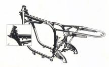
**BMW's frame** is a variable crosssection oval-tube cradle, light in weight, yet enormously strong. The crossing of the tubes at the steering head gives absolute torsional rigidity, while retaining the necessary longitudinal flexibility. The joints are welded by the reliable hydrogen-arc method used in the building of atomic reactors, a reflection of the overall quality of BMW. The rear wheel swing arm is supported by taper roller bearings, which hold it in perfect alignment.
