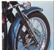
BMW's telescopic fork has hydraulic stops at full extension and compression. The long 8-inch travel of the front fork is tuned to the 5-inch rear suspension for unequalled roadability and riding comfort.
