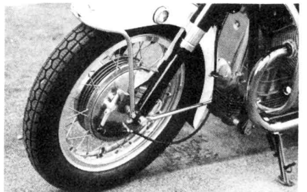
Guzzi front brake has dust cover over cable. Front end looked heavy.
