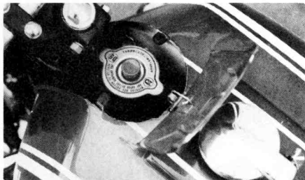
Suzuki's radiator filler is under cover on front of tank.
