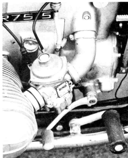
Sideways kickstarter locks out when ignition is off.
